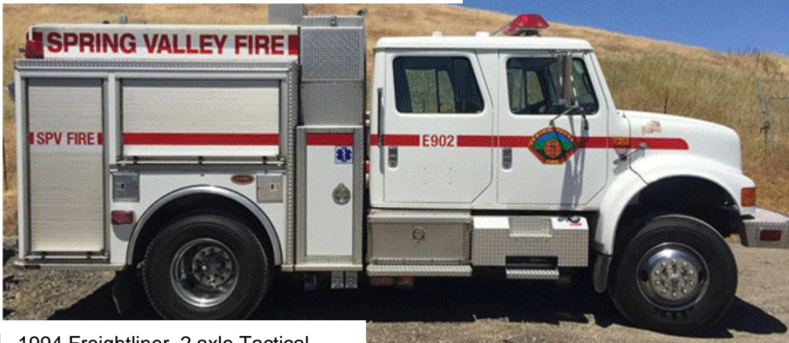
WT901 1994 Freightliner 2 axle Tactical water tender 2,000 gallons
