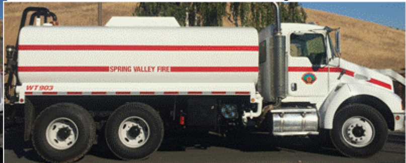
WT903 2005 Kenworth 3 axle water tender 3,900 gallons
